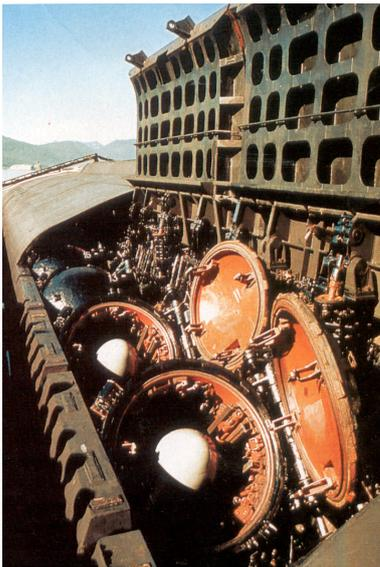
4 Starboard Missile Bank Forward - Silo Hatches Open
