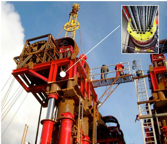
3 The strand jack (inset) mounted within the cable reel platform with the swell compensator rams underneath
